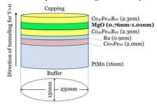
Structrures were annealed at 340°C in a magnetic field of 1 T. Next, the MTJs with 3 thickness of MgO barrier (0.76,0.95 and 1.01 nm) were patterned using electron-beam litography, ion-milling and lift-off processes. TMR values for the performed MTJs differs from 110% (0.76 nm MgO) to 170% (1.01nm MgO).
